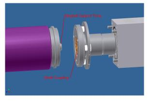
A non-bonded target assembly will require using the Lifting Collar, which is provided with a non-bonded target assembly, to guide the Magnet Support Tube into the Shaft Coupling.
