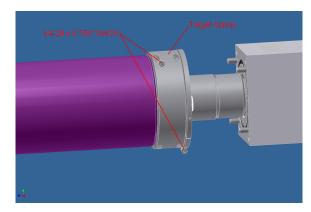
accept long <sup>1</sup>/<sub>4</sub>-28 SHCS to be used as points for tapping the 2 halves together with a mallet. These holes can also be used as jack-screw holes for removal of the Target Clamp.
