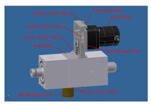
mount uprights. Now hold the motor securely and remove the 3/8-16 x 1.500" SHCS that is holding it in place. With the screw out, the motor can be taken off and set aside.
