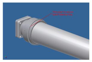
retaining rings by light bead blasting so they will resist flaking of the deposited target material.
