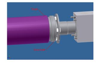
Drive Shaft may be stretched and need to be replaced. To do so, remove the Clamp Ring as shown in step 3 of the First Installation procedure above.
