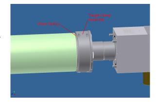
**NOTE:** When fully tightened, there should be roughly a 0.06" gap between the 2 halves. Try to keep this gap as evenly spaced as possible on both sides, although it does not need to be perfect.
