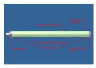
cannot be lifted by or supported on the tiles or they could break. Therefore, a Lifting Collar Assembly is bolted onto the open end of the Backing Tube in between the wave spring and Target Retaining Ring. This lifting collar has hooks on it so it can be suspended from a crane and handles for moving it by hand. The opposite end of the Target Assembly must be handled by the Support Nose. Take great care when installing a non-bonded target assembly so the target tiles do not break.
