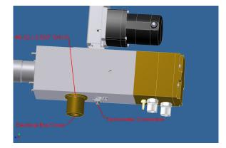
be necessary, refer to Addendum A for details. Also, the (2) #8-32 SHCS and the Electrical Bus Cover can be removed at this time.
