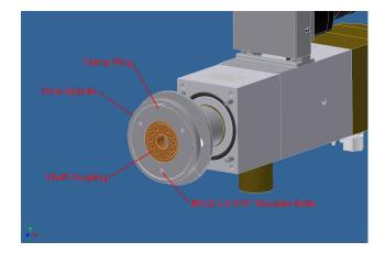
The Drive Spindle is held on with (8) #12-24 x 0.750" shes. Once these screws are removed, the spindle can be pulled off of the Drive Shaft. It may be a tight fit because of the double radial o-ring seal between the spindle and the shaft.
