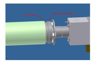
4. Now install the (2) Target Clamp halves on to the Target/Drive Shaft joint. The Target Clamp fastens together with (2) <sup>1</sup>/<sub>4</sub>-28 x 0.750" SHCS located diagonally from each other. Usually, the Clamps can be tapped directly in the center with a soft-faced mallet to seat them onto the Target and Drive Shaft. Or, opposite those holes are 2 counterbored, tapped holes that can
