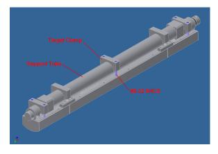
2. Insert the necessary shims as determined by analyzing the uniformity data and replace the Target Clamps and SHCS.
