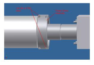
**NOTE:** For a non-bonded target assembly, the Lifting Collar will be required to support the drive side of the Target Assembly, as shown in the Target Mounting procedure above. Also, the opposite end must be handled by the Support Nose.
