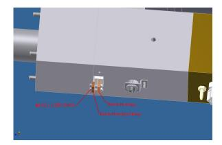
Clamp and insert the power cable and then tighten the clamp again. Also, a connection must be made between the cathode power supply ground or negative terminal and the chamber, which acts as the anode.
