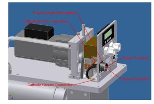
electrical connection. The receptacle and mating plug are rated for 120 Amps and there are (2) 4 AWG contacts. Be sure to use a cable that is rated to handle the maximum amount of power that will be applied. Multi-stranded and insulated copper wire is recommended.
