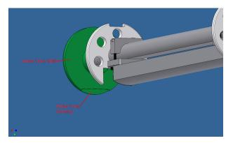
5. For reassembly of the Target on to the cathode, slide the Magnet Kit back into the Target and then follow the applicable Target Mounting procedure above. To check successful reassembly, perform the last step of the Target Mounting procedure. If necessary, the Target can be wiped clean at this time.
