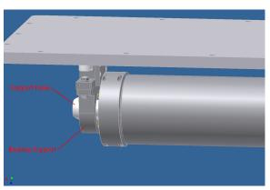
If it is difficult to engage the Support Tube into the Drive Shaft Coupling (Step 3, below), then it may be necessary to remove the Target End Cap on the Support Nose side by reversing Step 5 of the Target Mounting Procedure, described below. The Bearing Support will also need to be unbolted from its mounts by the (2) hex head bolts and nuts. The magnet pack and support tube can be slid out of the target tube to reduce the weight and make installation easier.
