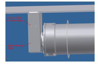
9. Attach a Debris Shield (Support Side) half to an Insulating Ring using (2) #10-32 x 0.375" low head SHCS. Do not fully tighten these screws until the other half and the retaining ring is on.
