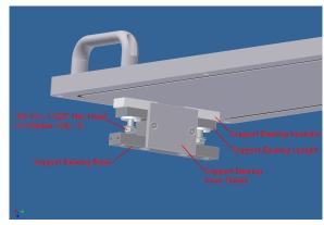
shown, with the inner shield facing the endblock. Be sure that the Support Bearing Insulators are aligned flush with the Inner Shield.
