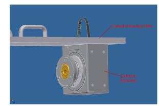
procedure. The first thing to do is check that the o-ring that seals to the chamber is clean as well as the o-ring groove and mating face. Next, the Endblock assembly can be lifted into place, aligning the mounting holes with the holes in the lid. This assembly will need to be supported here until it is bolted securely.
