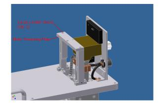
Attach the Drive Motor by making sure that the belt is on the drive pulley and then hold the belt up to slide the motor pulley inside of it. Lift the Motor up to remove the slack in the belt and place a 3/8-16 x 1.500" SHCS through the Motor Tensioning Plate and tighten it into the Motor Mount Plate until there is very little slack in the belt (it should appear tight at rest, but deflect about
