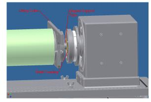
4. With the Target and Magnet Kit aligned, slide it into the Drive Shaft. Depending on the fit, you may need to push on the far end of the Target Assembly until the Backing Tube is seated inside of the Drive Shaft. A small amount of vacuum compatible grease may be applied to the inner lip of the Backing Tube to aid in installation. If it still cannot be assembled, then the o-ring in the
