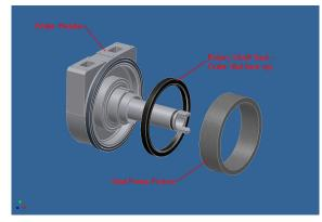
lubrication to safely use is **marine grease**. This lubricant is water compatible and will offer a longer service life than vacuum compatible or standard grease.
