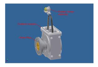
Also, the Rotation Sensor Assembly needs to go back on using the (2) #8-32 x 0.500" SHCS.
