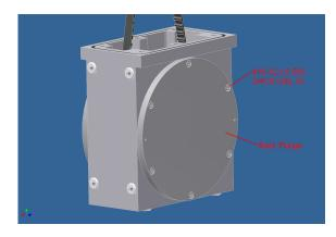
8. Next, use (2) of the #10-32 x 0.500" SHCS as jack-screws to evenly back out the Water Header and Drive Shaft Assembly. Once it is out far enough, it will easily pull out by hand. Slip the Belt off of the Drive Pulley and take it out of the top of the Endblock.
