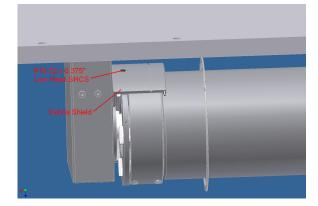
10. Attach the other Debris Shield (Support Side) to the Insulating Ring with (2) #10-32 x 0.375" low head SHCS. You must align the pins in the ends of the Shields in order for them to fit together. Then snap the Debris Shield Retaining Ring into place in the groove in the Debris Shield halves.
