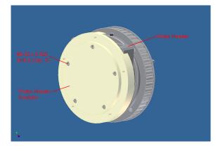
12. Now the Water Header Assembly can be pressed out of the Drive Shaft Assembly. But first the #6-32 x 0.250" SHCS needs to be removed from the Water Header in order for the assemblies to come apart easily (since the screw is located between (2) rotary seals, it creates an air pocket between them).
