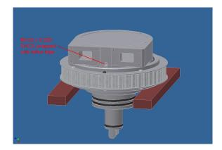
19. The Rotary Shaft Seals on the Vacuum Seal Assembly can now be serviced. Use a small blade screwdriver to remove the retaining ring that holds the rotary seals in place.
