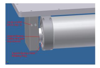
7. Place the Upper Shield Ring on the Lower Shield Ring, line up the retaining ring groove and then snap the retaining ring into place. A screwdriver may be needed to slide the retaining ring into the groove, as there isn't much room for hands.
