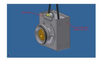
Take off the Tachometer Sensor Assembly by removing the (2) #8-32 x 0.500" SHCS and lifting the assembly out of the Endblock.
