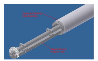
4. When reinstalling the magnet tube be sure that the Water Drain Baffle opening is facing down.
