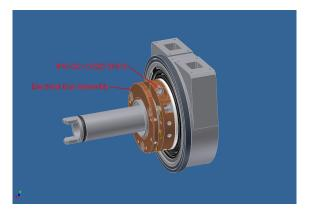
14. Now slide off the Front Seal Spacer, the inner Rotary Shaft Seal and the Back Seal Spacer.
