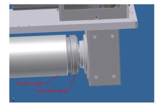
in the Drive Shaft may be stretched and need to be replaced. Refer to Steps 4-5 in the Rotary Seals Maintenance Procedure to do so.
