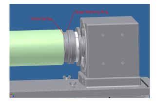
5. Now install the (2) Target Clamp halves on to the Target/Drive Shaft joint. The Target Clamp fastens together with (2) 8-32 x 0.750" SHCS located diagonally from each other. Usually, the Clamps need to be hit directly in the center with a *soft-faced mallet* to seat them onto the Target and Drive Shaft.
