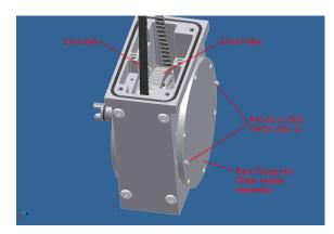
9. The Vacuum Seal Assembly is then removed by taking out the (6) # 10-32x 0.500" SHCS out of the Front Flange and then sliding the assembly out of the Endblock.
