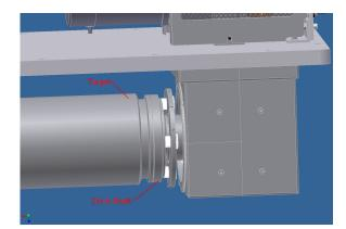
Drive Shaft may be stretched and need to be replaced. Refer to Steps 4-5 in the Rotary Seals Maintenance Procedure to do so.
