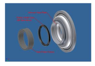
**NOTE:** These rotary seals are sealing between atmosphere and vacuum, so they must be lubricated with **Tribolube-15**, which is vacuum compatible (*do not use marine grease on these seals*).
