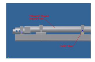
4. The Magnet Kit and Support Tube can now be installed back into the target tube assembly. After that, the Magnet Kit to target tube assembly clearance can be checked by rotating the Target (or Magnet Kit and Support Tube) and listening for any rubbing of the Magnet Kit on the inside of the Backing Tube. If no rubbing is detected, it is acceptable to run the target. Otherwise, shims must be removed until clearance is achieved between the Magnet Kit and Backing Tube.
