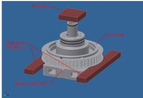
Note the (2) locations for supporting the Drive Shaft Assembly are on the Drive Shaft itself, not on the pulley.
