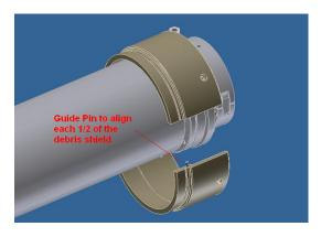
5. For reassembly of the debris shields onto the target assembly, reverse the procedures 1-4 above. To check successful reassembly, use an ohm-meter to check conductivity between the debris shield and the target surface. This should be an OPEN (no contact) circuit. Check each debris shield also to the chamber or system ground. This also should be OPEN circuit.
